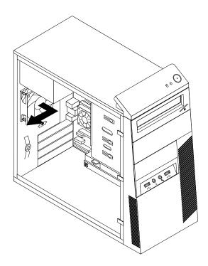
Figure 43. Removing the rear fan
